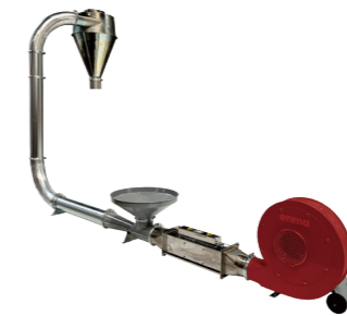
EnMa CP-B Positive pressure blowing device The crushed material will be blown to the designated position through the fan blower. The materials with more strict requirements will not pass through the fan impellers, which avoids the pollution and impact of the materials.
