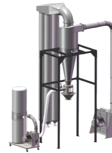
EnMa CP-A Positive pressure suction device The crushed material can be absorbed into the cyclone through the fan blower, and the dust can be separated through the work of the cyclone. If the dust removal effect is not achieved, the dust collector of ENMA brand can be increased to further dust removing.
