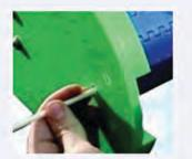
The easy change belt system makes the conveyor extremely versatile and removing the belt is simple. By extracting a single pin, the belt can be completely removed from the conveyor framework which allows links to be taken out to compensate for belt stretch. If necessary damaged links can be replaced or flight bands can be added or removed (as shown).
