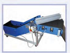
**ROTARY BOX FILLER** Rotary Box Fillers are the ideal solution for product distribution into multiple boxes. Up to 10 box positions can be programmed with easy set up control.
