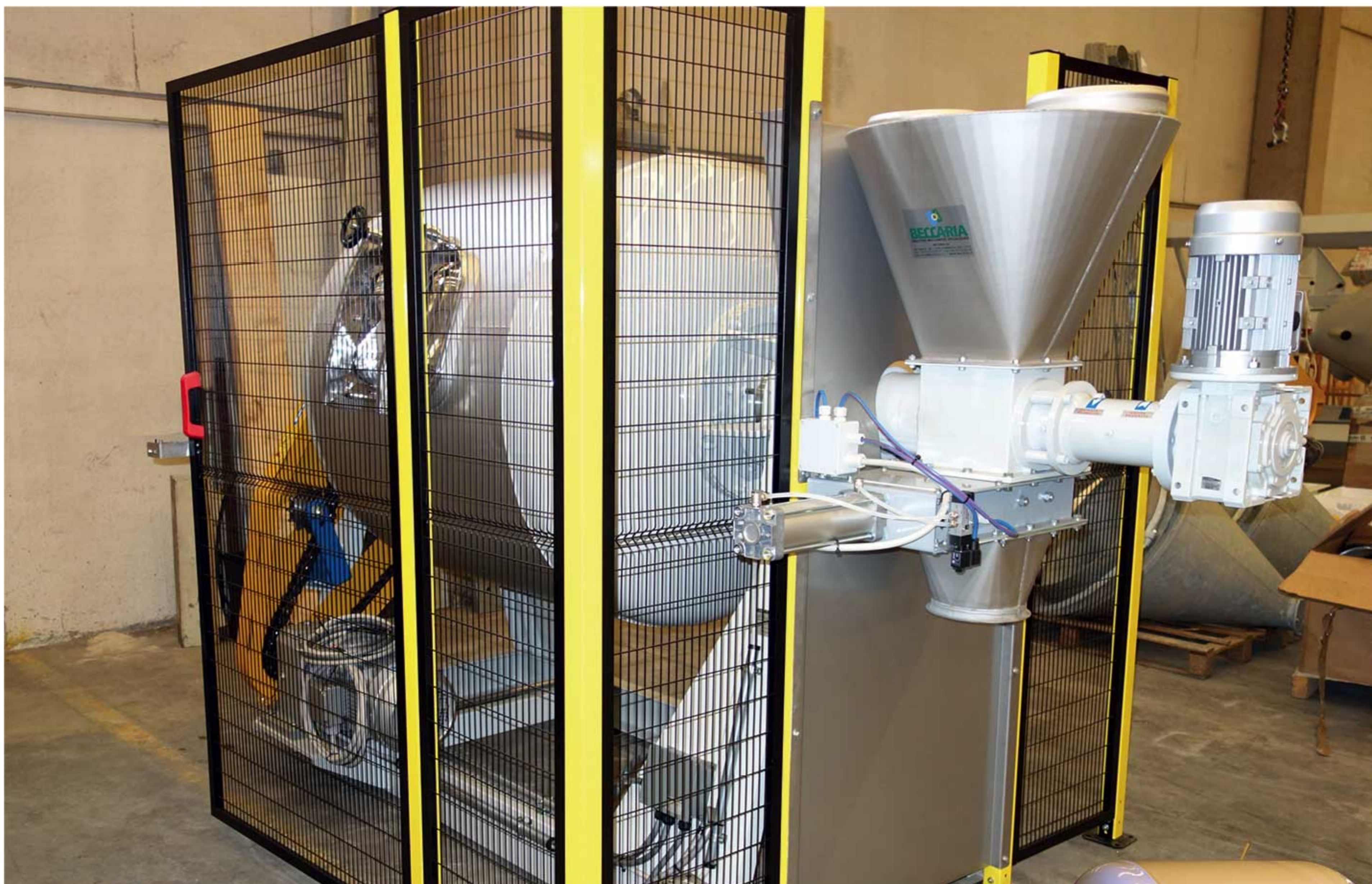
Mix BROV Litri 1000 in acciaio INOX BROV mixer Liters 1000 made of stainless steel
