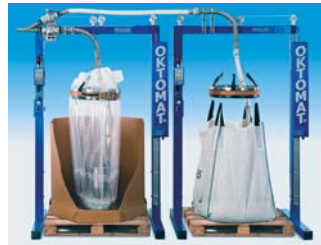
OKTOMAT® twin station with automatic switch-over
