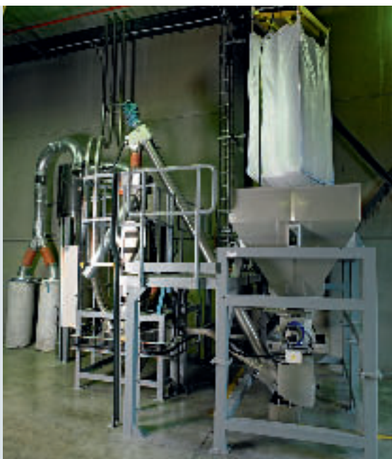
Big bag unloading unit with flake dedusting unit
